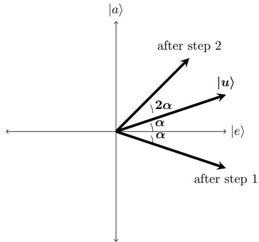
Figure 2: Step 2 - Reflecting around  $|u\rangle$
